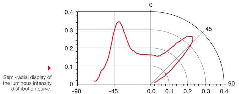
Semi-radial display of the luminous intensity distribution curve.
